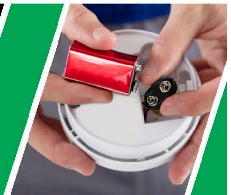
9-volt alkaline battery smoke alarm
