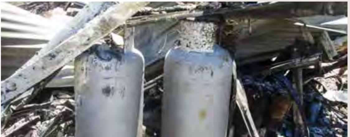
Below: LP gas cylinders stored under a house—Roleystone 2011.
